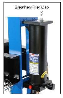
2. Open the release valve by turning it counterclockwise. Pump five to ten full stokes until the handle regains a firmer feel.
