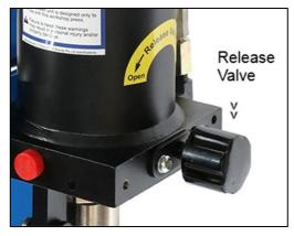
3. Close the release valve and Insert the Pump Handle into the socket of manual pump and pump the handle until the ram is at full stroke.
